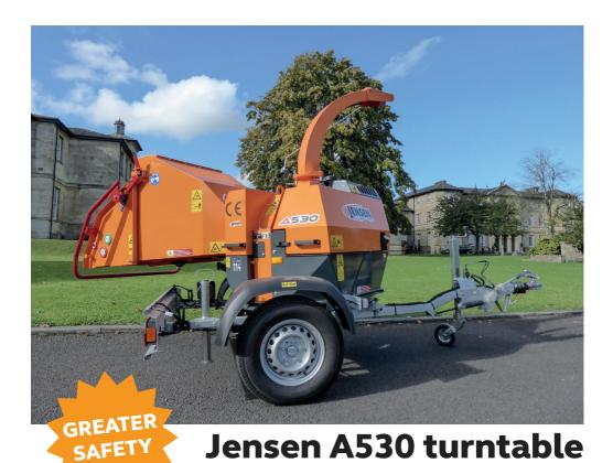
The new A530 turntable from Jensen saves you time, effort and money. With the ability to turn the chipper up to 270 degrees, you can load the machine from a range of angles and directly from the verge whilst the 270 degree rotating chute disposes of the chippings in your preferred direction.
